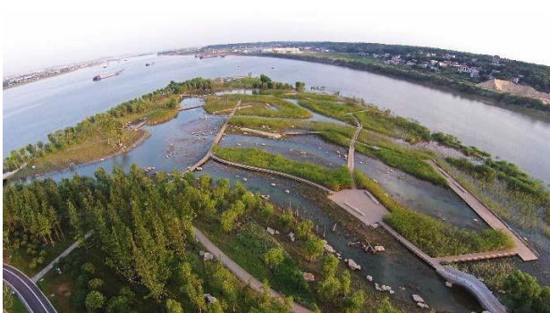
Variable grading makes the flood fluctuation no longer a threat, offering instead an opportunity for increasing biodiversity. Different water levels contribute to various habitats. This image shows the south wetland in summer with high water level.
